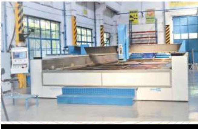
5 Axis CNC Water Jet Cutting Facility
