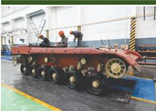
Assembly of Tank T85UG
