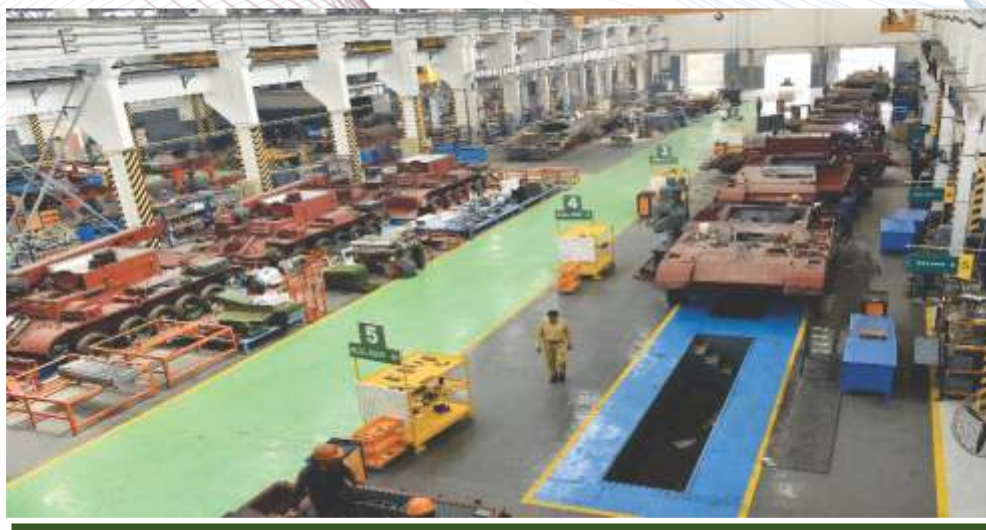
Assembly Shop - Tank T85UG & ARVs
