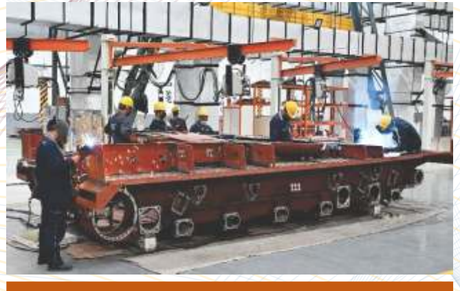
Welding of Armoured Plates - Tank Hull
