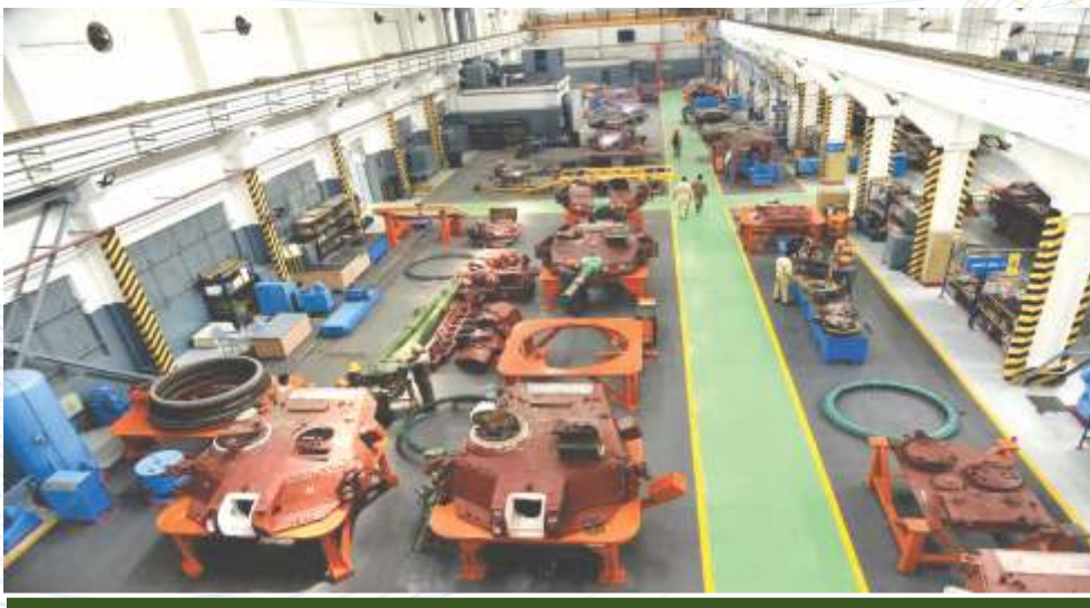
Turret Assembly Shop - Tank T85UG / ARVs
