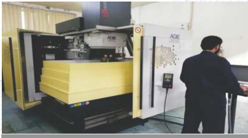
EDM Wire Cut Facility
